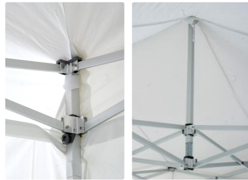
STEP 2: Fit roof. Fit corners of roof to corners of frame. Fit centre of roof pocket over centre post.
