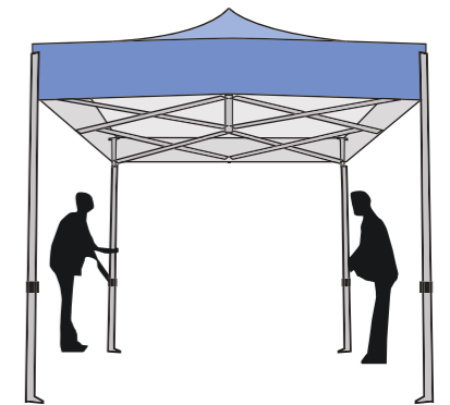
STEP 6: Extend legs to desired height. Ensure locking pins have engaged.
